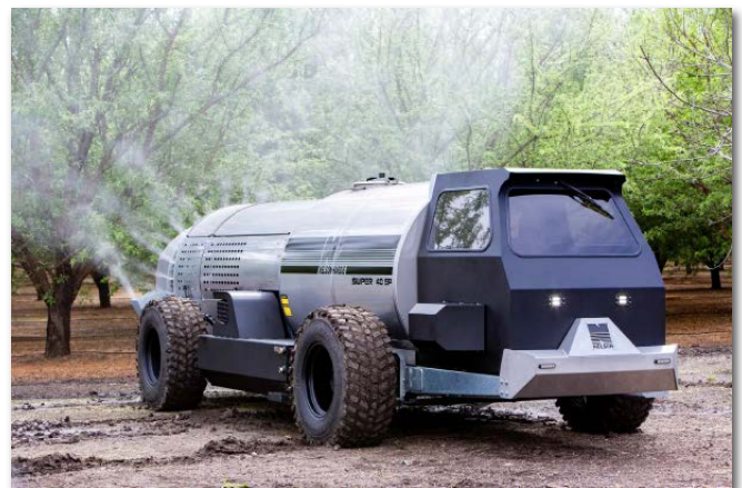
The Neslon Hardie Super 40SP features 4-wheel steering and drive. (photo courtesy of Nelson Mfg.)
